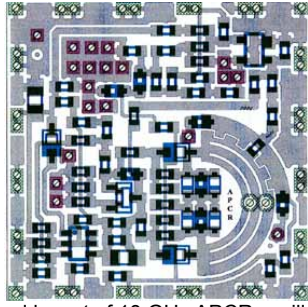
Fig. 14. A typical layout of 18 GHz APCR oscillator using ATI
